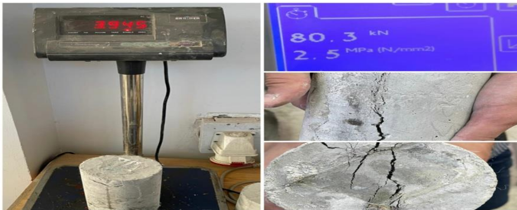
Figure 4-33 : Cylinder Tensile test (After 28 Days). Sixth Mix
