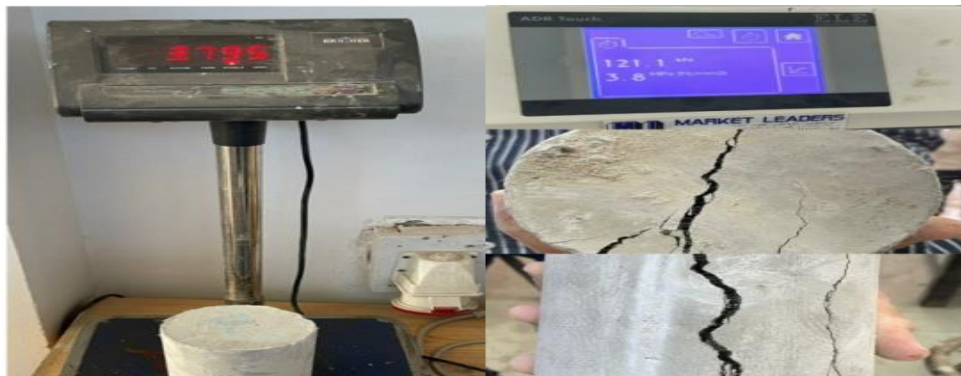
Figure 4-29 : Cylinder Tensile test (After 28 Days). Second Mix
