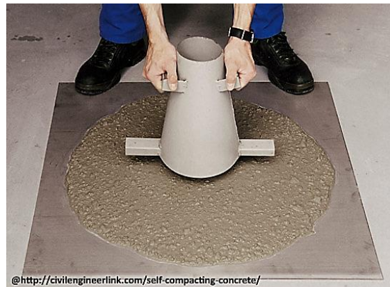
Figure 2-10: High fluidity and flow are the most important characteristics of self-compacting concrete
