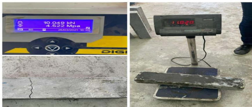
Figure 4-38 : Flexural Strength test (After 28 Days). Second Mix
