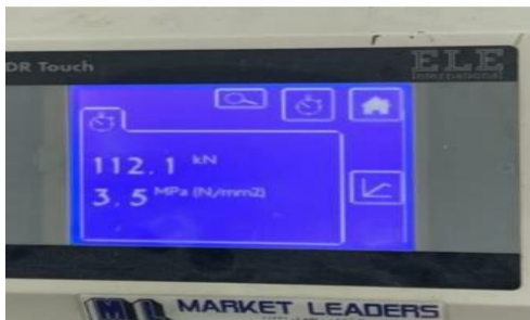
Figure 4-28 : Cylinder Tensile test (After 28 Days). Second Mix
