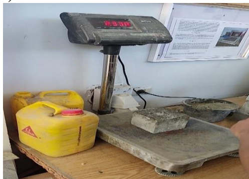
Figure 4-17 : Cube compressive test (After 7 Days). ninth Mix
