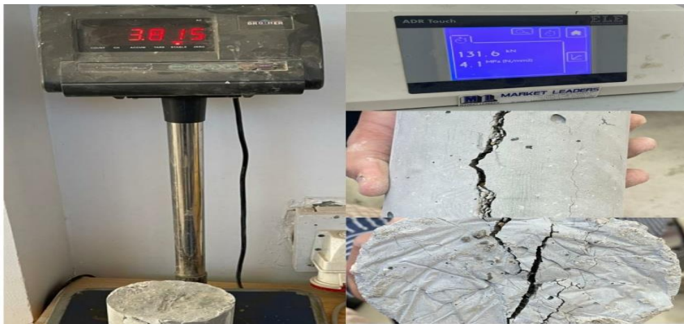
Figure 4-31 : Cylinder Tensile test (After 28 Days). Fourth Mix
