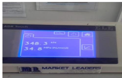
Figure 4-25 : Cube compressive test (After 28 Days). Eighth Mix
