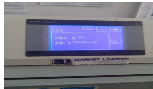
Figure 4-23 : Cube compressive test (After 28 Days). Sixth Mix
