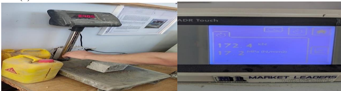
Figure 4-15 : Cube compressive test (After 7 Days). Seventh Mix
