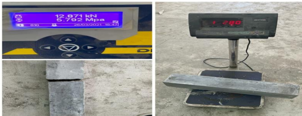
Figure 4-45 : Flexural Strength test (After 28 Days). Sixth Mix
