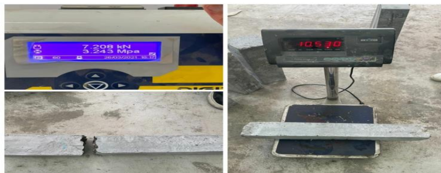
Figure 4-37 : Flexural Strength test (After 28 Days). First Mix
