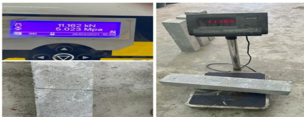
Figure 4-44: Flexural Strength test (After 28 Days). Eighth Mix
