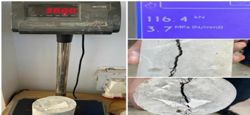
Figure 4-35 : Cylinder Tensile test (After 28 Days). eighth Mix
