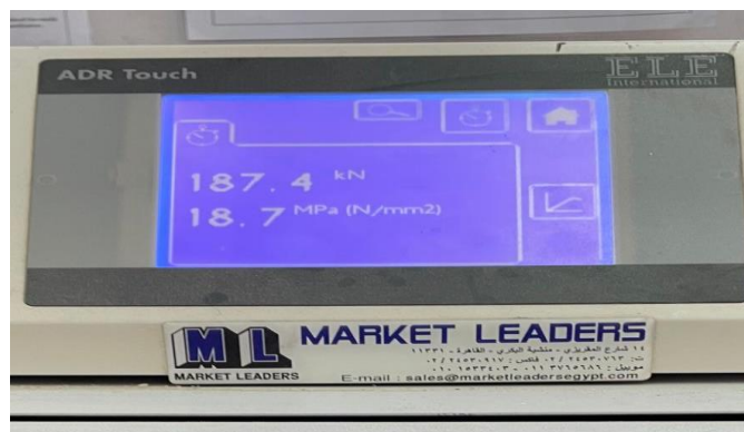
Figure 4-10: Cube compressive test (After 7 Days). Second Mix
