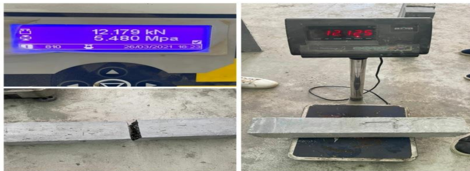
Figure 4-40 : Flexural Strength test (After 28 Days). Fourth Mix
