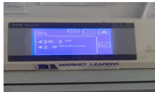
Figure 4-22 : Cube compressive test (After 28 Days). Fifth Mix
