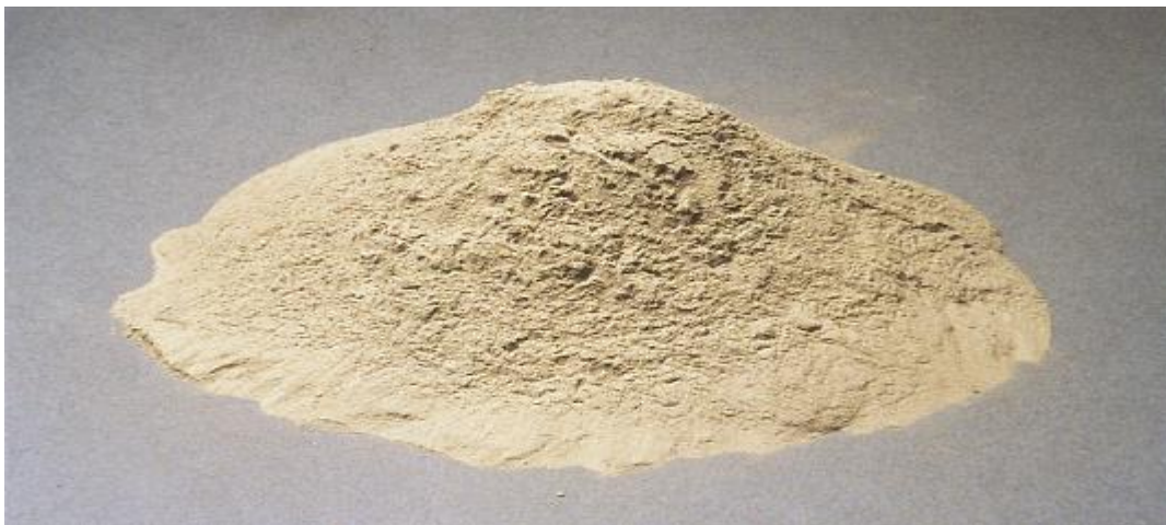
Figure 3-8: Fly ash, a powder resembling cement, has been used in concrete since the 1930.
