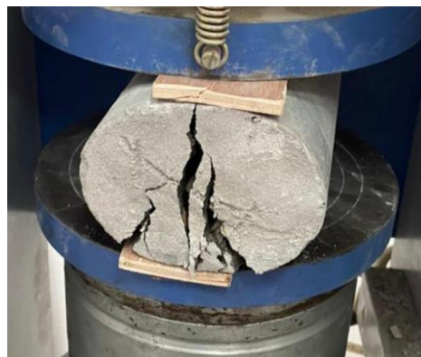
Figure 4-27 : Cylinder Tensile test (After 28 Days). First Mix
