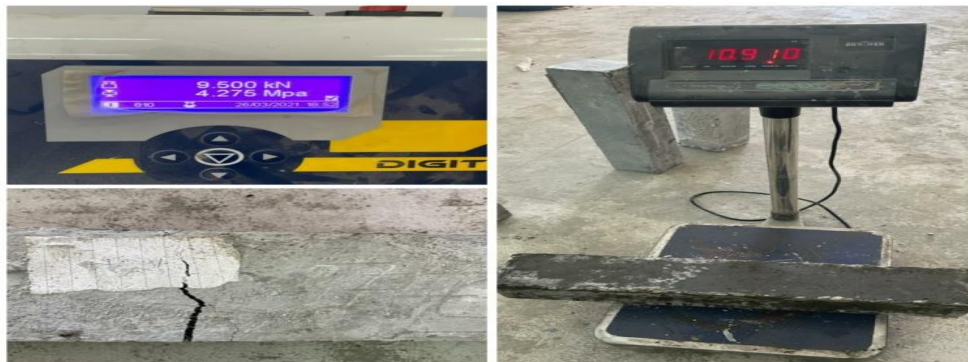
Figure 4-43 : Flexural Strength test (After 28 Days). Seventh Mix
