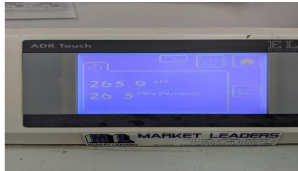
Figure 4-11 : Cube compressive test (After 7 Days). Third Mix
