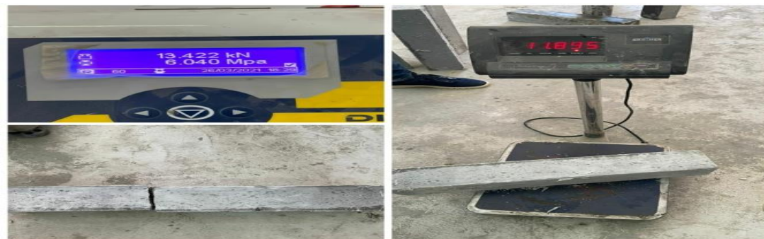
Figure 4-41 : Flexural Strength test (After 28 Days). Fifth Mix
