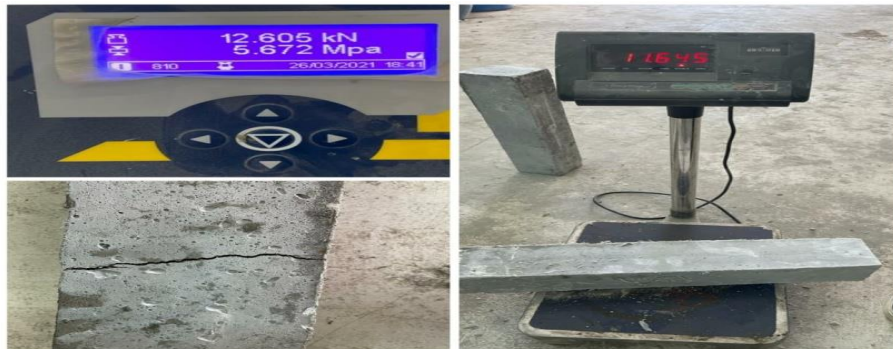
Figure 4-39 : Flexural Strength test (After 28 Days). Third Mix
